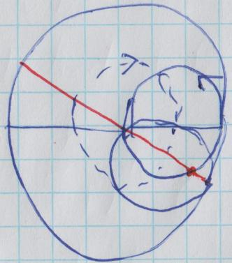
Have a small circle rolling inside a circle of twice the diameter. Each point on the outside of the small circle traces out a diameter of the larger one, moving back and forth along that diameter.
