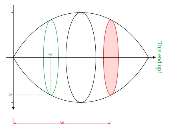
The tank is completely filled with water which is then drained from the tank at a contant rate of 100 litres per minute. Suppose that a given instant the water in the tank is w metres deep.
