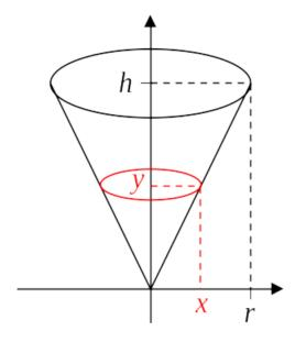
makes it evident that when the piece of arc at x is revolved about the y-axis, it goes around a circle of radius R = x - 0 = x. Since  $0 \le x \le r$  for the piece of the line  $y = \frac{h}{r}x$  which gets revolved to make the cone, it follows that the surface area of the cone, not counting the blunt end, is given by:
