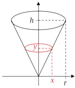
For the region being revolved to make the cone, *i.e.* the region between y = 0 and  $y = \frac{h}{r}x$  for  $0 \le x \le r$ , we have  $0 \le y \le h$ . The disk at y has radius  $R = x - 0 = x = \frac{r}{h}y$ , so this disk has area  $\pi R^2 = \pi \left(\frac{r}{h}y\right)^2 = \pi \frac{r^2}{h^2}y^2$ . It follows that the volume of the come is given by:
