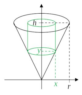
As is evident from the diagram above, the shell at x, for some x with  $0 \le x \le r$ , has radius R = x - 0 = x and height  $H = h - y = h - \frac{h}{r}x = h\left(1 - \frac{x}{r}\right)$ , and hence has area  $2\pi RH = 2\pi xh\left(1 - \frac{x}{r}\right) = 2\pi h\left(x - \frac{x^2}{r}\right)$ . It follows that the volume of the come is:
