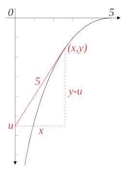
Suppose the sled is at (x, y) at the instant that the dog pulling the sled is at (0, u). The tether is then the hypotenuse of a triangle with vertices at (x, y), (0, u), and (x, u),
