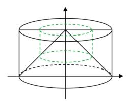
Since we revolved about the y-axis, the shells are vertical and we ought to use x as the basic variable. The shell at x has radius r = x - 0 = x and height h = 4 - y = 4 - (4 - x) = x, so it has area
