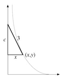
By the Pythagorean Theorem,  $c^2 + x^2 = 3^2$ , so  $c = \sqrt{3^2 - x^2} = \sqrt{9 - x^2}$ . The slope of the leash – which is equal to  $\frac{dy}{dx}$  because the leash is tangent to the curve – is then  $\frac{\text{rise}}{\text{run}} = \frac{-c}{x} = -\frac{\sqrt{9 - x^2}}{x}$ . (Note that the slope must be negative because the leash goes down from left to right.) It follows that  $f'(x) = \frac{dy}{dx} = -\frac{\sqrt{9 - x^2}}{x}$ .
