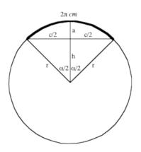
We'll need some of the fundamental relationships among the various items mentioned in the diagram. First, note that, in a circle of radius r, the length of the arc subtended by an angle of  $\alpha$  radians — that is, the length of the hair — is just  $r\alpha$ . (This simplicity is one of the pleasant benefits of using radians.) In our set-up, this means that
