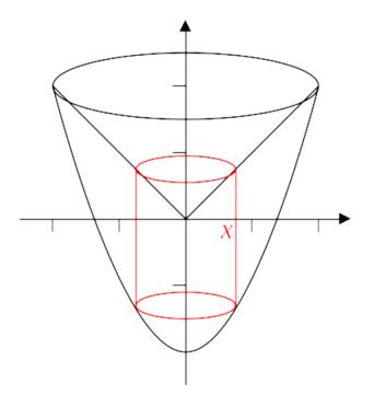
Note that since we are using cylindrical shells for our "cross-sections", we should use the variable, in this case x, whose axis is perpendicular to the axis of revolution. The shell at x, where  $0 \le x \le 2$ , has radius r = x - 0 = x and height  $h = x - (x^2 - 2) = -x^2 + x + 2$ , and hence has area  $A(x) = 2\pi r h = 2\pi x (-x^2 + x + 2) = 2\pi (-x^3 + x^2 + 2x)$ .
