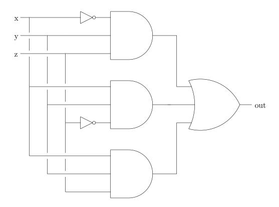
Figure 2.5: A digital logic circuit built using disjunctive normal form. The output of this circuit is  $(\neg x \land y \land z) \lor (x \land y \land \neg z) \lor (x \land y \land z)$ .
