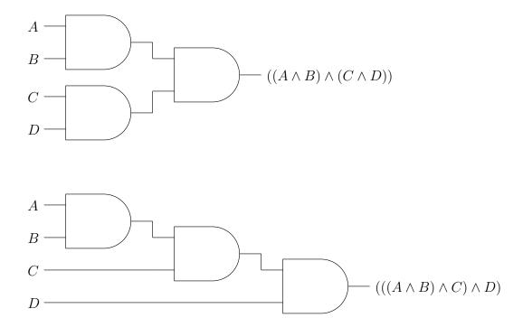
Figure 2.4: Two of the possible ways to parenthesize the conjunction of four statement variables – expressed as digital logic circuits.
