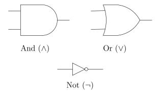
An and-gate has two transistors inside it that are wired in series – if both the inputs are energized the output will be too. An or-gate has two transistors in parallel inside it. Not-gates involve magic – when their input is not on, their output *is* and vice versa.
