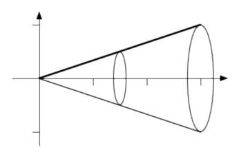
We will find the volume of the solid by using the disk/washer method. Since we obtained the solid by revolving the region about a horizontal line, namely the x-axis, we will need to integrate with respect to x using the limits 0 to 3 given by the original region. For each x, the cross-section is a washer with outside radius  $R = y - 0 = \frac{1}{3}x$  and inside radius r = 0 - 0 = 0. Thus the volume of the solid is:
